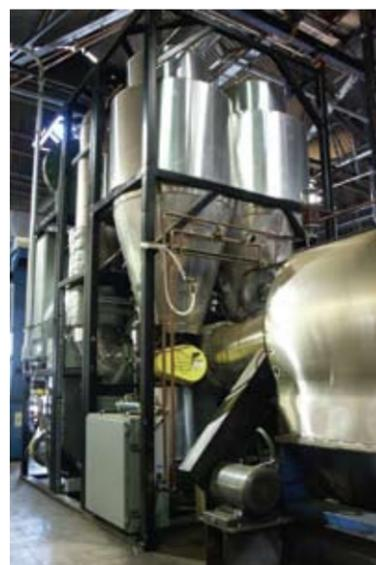
A roaster at Hawaii Coffee Company showing a recirculating system attached to the back of a 23R Jabez Burns roaster. The two bullet-shaped cyclones manage increased airflows.
